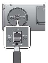
\* Do not connect your mobile device to the USB port and the Docking station at the same time for recharging.
